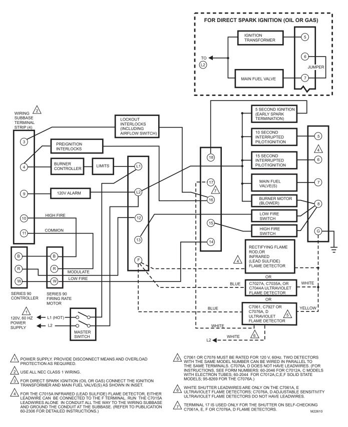
Fig. 12. Sample block diagram of field wiring for the R7140L1009, used for replacing R4140L Programmers with pre-ignition interlocks.
