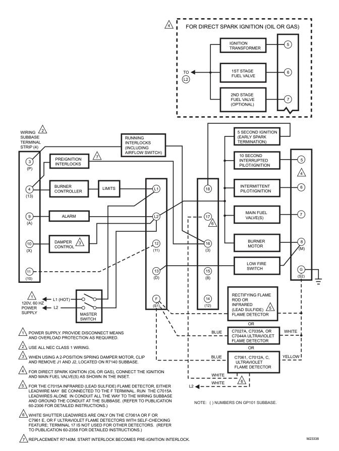
Fig. 18. Block diagram of field wiring for the R7140M1007, used for replacing R4140M Programmers with Pre-Ignition Interlocks.
