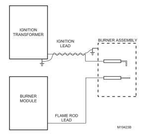
Fig. 20. Eliminating ignition interference.
