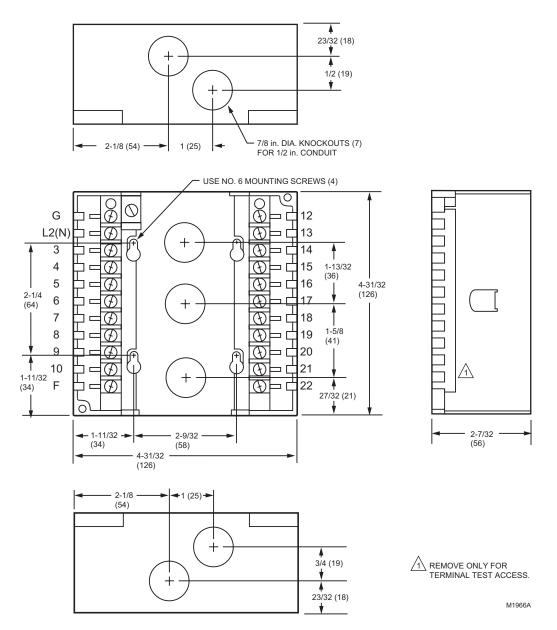
Fig. 2. Top and front view of Q7800B1003 Wiring Subbase (4-sided) with dimensions in in. (mm).
