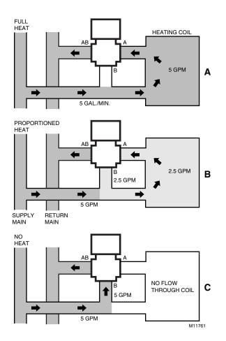
Fig. 8. Three-way mixing valve operation–coil bypass. Three-way valves maintain constant flow in the piping. As the temperature requirements change, the volume of the fluid in the coil varies.
