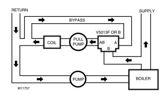
Fig. 4. Typical V5013F or B mixing valve with constant volume through coil.
