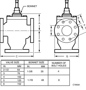
Fig. 1. V5013B,C Flanged Body Dimensions.
