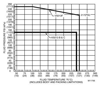
Fig. 3. Valve pressure-temperature ratings.
