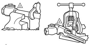
USE PROPERLY REAMED AND CLEANED PIPE AND MODERATE AMOUNT OF DOPE (LEAVE TWO THREADS BARE).
