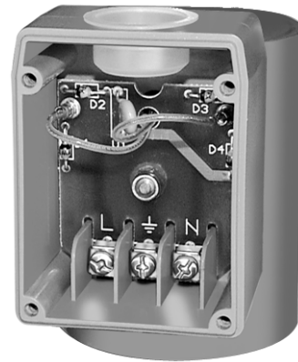
Fig. 12. Wiring compartment of V4297A SSOV.
