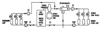
**Multiple Loops** 2.1.2 Each loop operates at different temperature.
