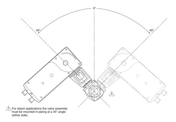
Figure-16 Typical Mounting Position for Steam Applications.
