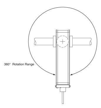
Figure-17 Actuator Positioned Anywhere Within 360 Degrees.
