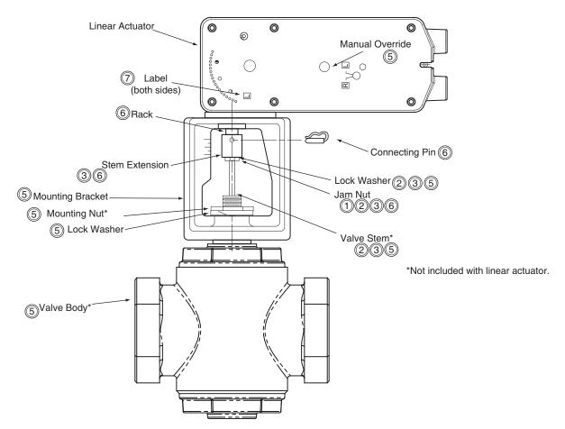
Figure-13 Typical Assembly and Installation.
