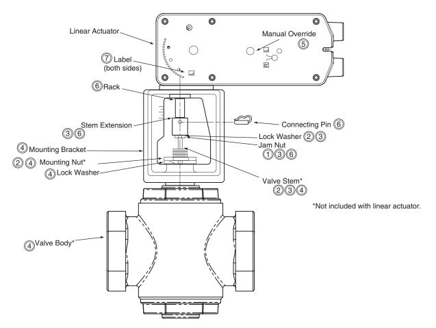
Figure-14 Typical Assembly and Installation.
