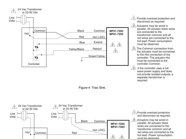
Figure-5 Triac Sink With Separate Transformers.
