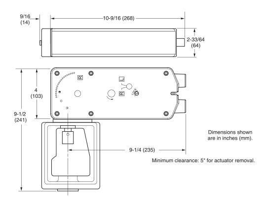
Figure-20 Mx61-720x Spring Return Valve Actuator Dimensions.
