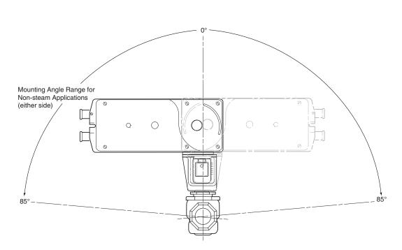
Figure-15 Typical Mounting Position.
