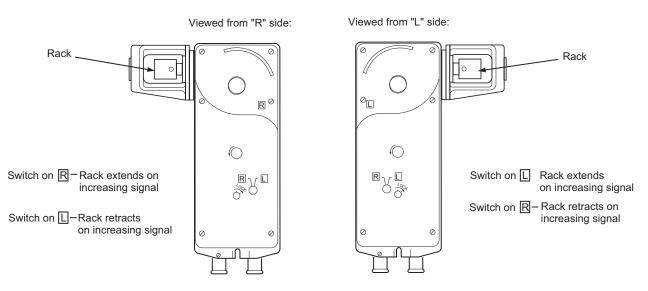
Figure-9 Rotation Switch Settings for MSx1-7203 Proportional Actuators.
