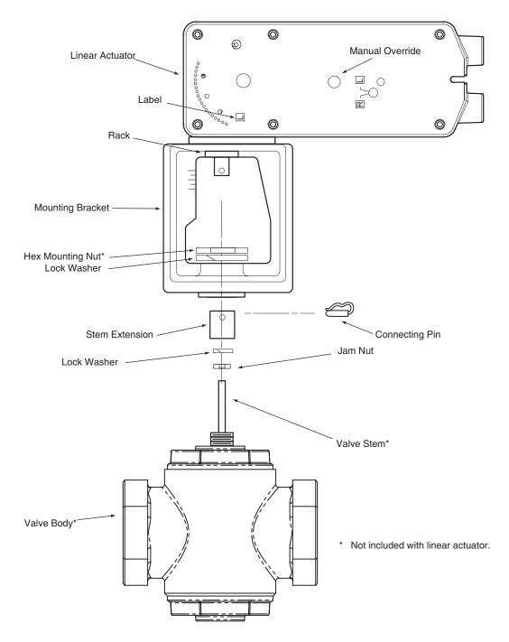
Figure-12 Mx61-720x Series Actuator Exploded View.
