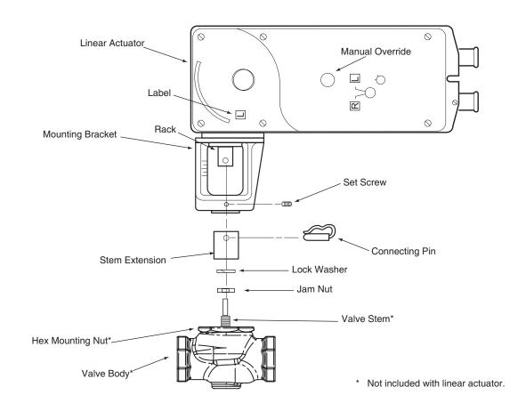
Figure-10 Mx51-720x Series Actuator Exploded View.
