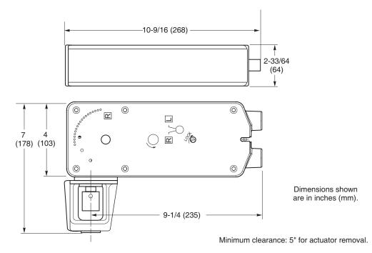
Figure-19 Mx51-720x Spring Return Valve Actuator Dimensions.
