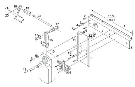
Figure 1: Damper Mount Linkage Kit, in./mm
