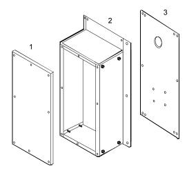
Figure 5: Weathershield Enclosure
