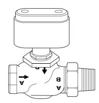
Figure-4 MK-2690 Actuator Mounted on VB-7XXX Valve.
