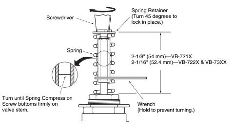
Figure-3 Installation of Linkage Spring.
