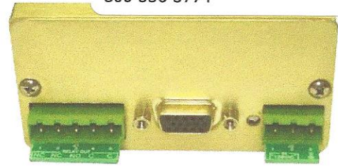
Rear View of 5004-216RN shows remote reset terminal block, 12-pin connection display cable connect, and power input terminal block
